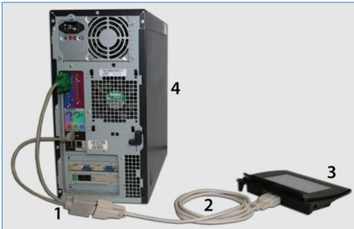
1. Y-cable adapter (included in Topaz Serial Cable Kit) connected from the serial extension cable to the computer's serial port (for pad communication) and the computer's USB port (for power)
