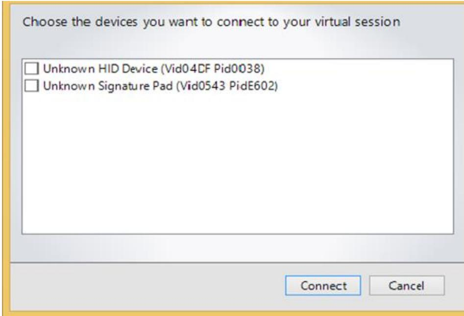
Check the “Unknown Signature Pad (Vid0543 PidE602)” item, then press the “Connect” button. On the VDA Tool Bar, the Devices tab shows the GemView Tablet Display connected with a check mark before the name.
