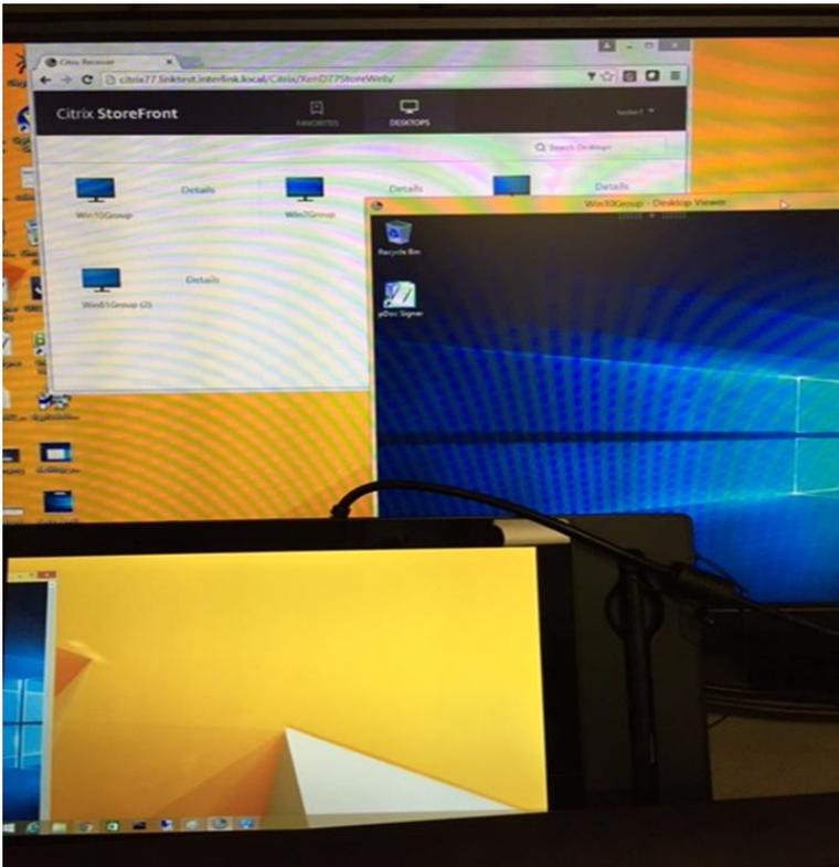
Press the “Maximize” button on the Citrix Desktop Viewer window on the Gem View Tablet Display, as the following photo shows:
