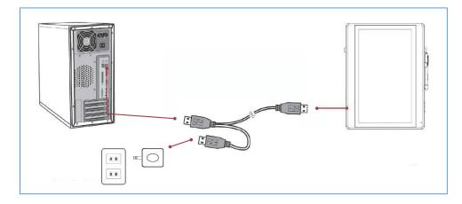
**Note:** Connect both USB connectors at one end of the cable to the PC, to ensure a stable power supply. Due to the manner that Windows enumerates USB devices and the use of internal USB hubs in some PCs, it may be necessary to change the ports into which the USB connectors are inserted.
