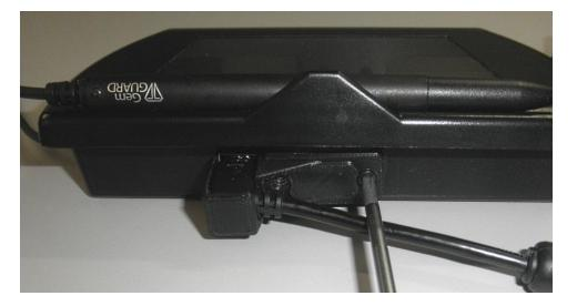
4. Re-attach the vertical pen holder removed in step 2.
