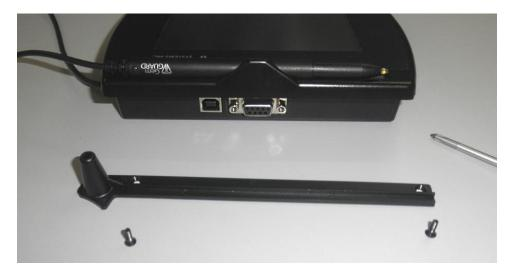
2. Put the USB cable into the strain relief bracket and plug back into the pad.
