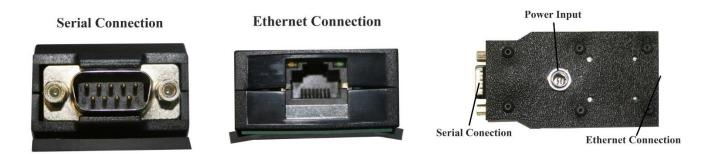
Once the power supply, Topaz pad, and ethernet cable (also connected to the Network Hub) is connected, an orange light (for network connection) and blinking green light (for power) should be visible, denoting the ethernet adapter is functioning.
