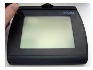
A small line of dots will appear in the upper left corner of the LCD screen. While holding the pen at a natural writing angle, lift pen tip from display, press pen tip back down on the upper left most dot and hold.
