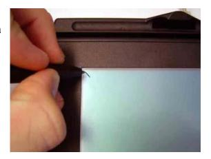
3. The mark will disappear from the upper left corner, and reappear in the lower right corner. Press pen tip on lower right dot and hold.
