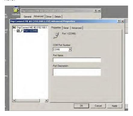
It is important to note though that changing the COM port setting after installation will require that the SigPlus.INI file be altered either manually or through <u>SigPlus Adjust</u>.
