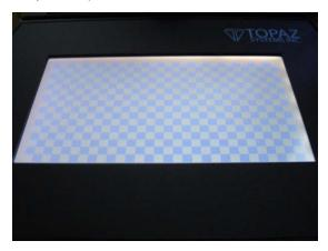
In order to test writing a string to your LCD, use the LCD WriteString Test. You can customize the font, size, and text of the message displayed.
